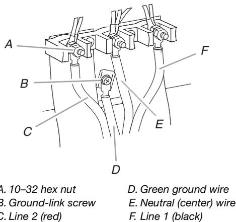
6. Connect line 2 (red) and line 1 (black) wires to the outer terminal block posts with 10–32 hex nuts.
