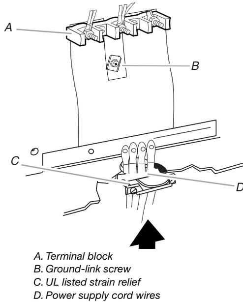
4. Use a Phillips screwdriver to connect the green ground wire from the power supply cord to the range with the ground-link screw and ground-link section. The ground wire must be attached first.
