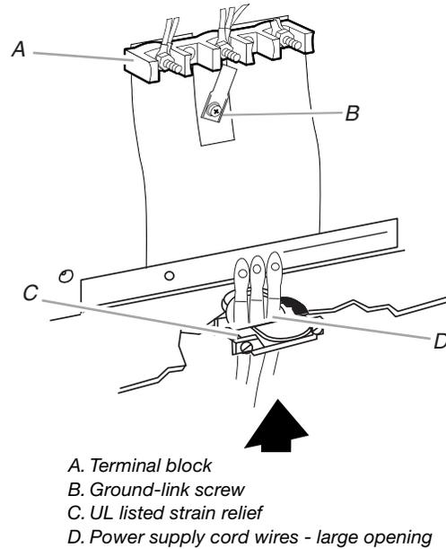
2. Use  $\frac{3}{8}$ " nut driver to connect the neutral (white) wire to the center terminal block post with one of the 10–32 hex nuts.
