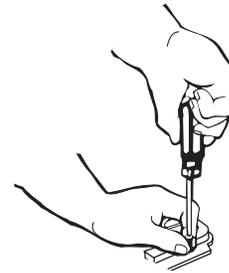
Depending on the thickness of your flooring, longer screws may be necessary to anchor the bracket to the subfloor. Longer screws are available from your local hardware store.
