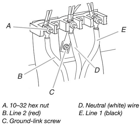
3. Connect line 2 (red) and line 1 (black) wires to the outer terminal block posts with 10–32 hex nuts.
