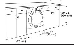
For closet installation, with a door, the minimum ventilation openings in the top and bottom of the door are required. Louvered doors with equivalent air ventilation openings are acceptable.
