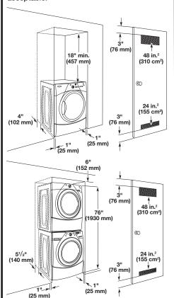
For cabinet installation, with a door, the minimum ventilation openings in the top are required.
