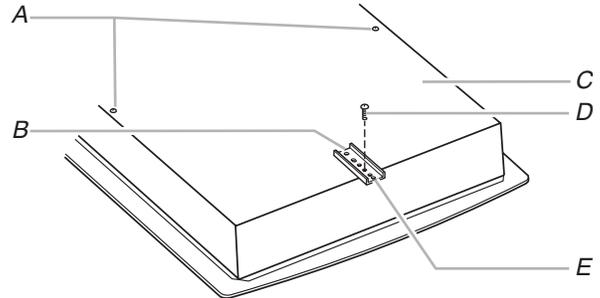
A. Attachment screw holes for optional front and back location
