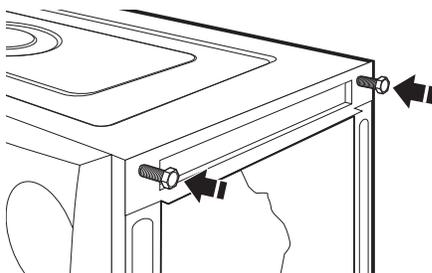
5. Slide the pedestal onto the All-In-One Washer and Dryer by engaging the bolts in the slots located on the top of the pedestal.
