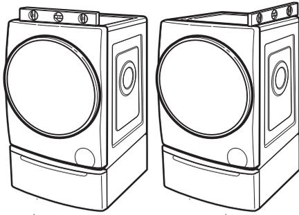
10. Adjust the feet so that the rubber pads extend just below the bottom of the pedestal and keep the pedestal at least 1/8" (3.175 mm) off the floor.
