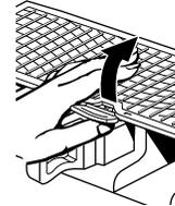
**NOTE:** Be sure the cover is completely latched before pulling out the bottom rack and before closing the dishwasher door.
