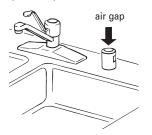
that the drain hose either be looped up and securely fastened to the underside of the counter, or be connected to an air gap. Make sure to use an air gap if the drain hose is connected to house plumbing lower than 20" (50.8 cm) above subfloor or
