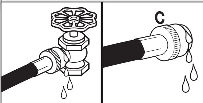
Turn on water faucets to check for leaks from faucet and at washer connection. A small amount of water may enter washer. You will drain this in a later step.
