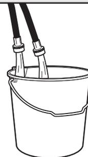
Run water for a few seconds through hoses into a laundry tub, drainpipe, or bucket to avoid clogs. Water should run until clear. Check the temperature of the water to make sure that the hot water hose is connected to the hot water faucet and the cold water hose is connected to the cold water faucet.
