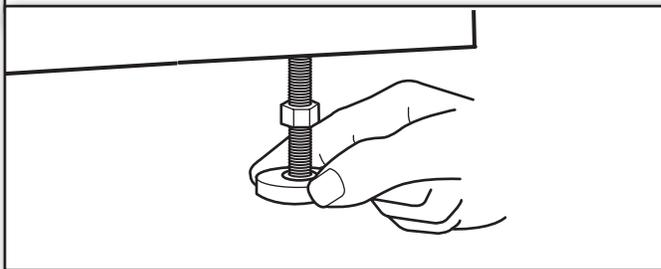
For washers with an adjustable right front foot, lower the right front foot until it contacts the floor. Using pliers, rotate the foot up to an additional 1 1/2 turns.
