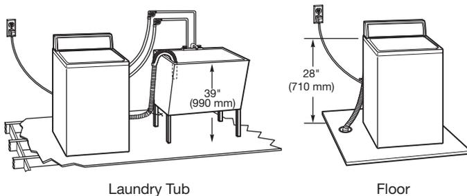
The laundry tub drain system needs a minimum 20 gal. (76 L) capacity laundry tub. The top of the laundry tub must be at least 39" (990 mm) above the floor and no higher than 96" (2.4 m) from the bottom of the washer.
