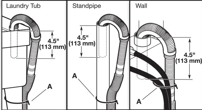
Secure drain hose to laundry tub leg, drain standpipe, or inlet hoses for wall standpipe with removable tie strap (A). This will help reduce the chance of drain water splashing on the floor.
