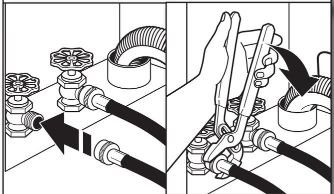
Make sure the washer basket is empty. Attach the hose labeled hot to hot water faucet. Screw on coupling by hand until it is seated on washer. Use pliers to tighten couplings an additional two-thirds turn. Repeat this step with the hose labeled cold for the cold water faucet. Both hoses must be connected for washer to work properly.
