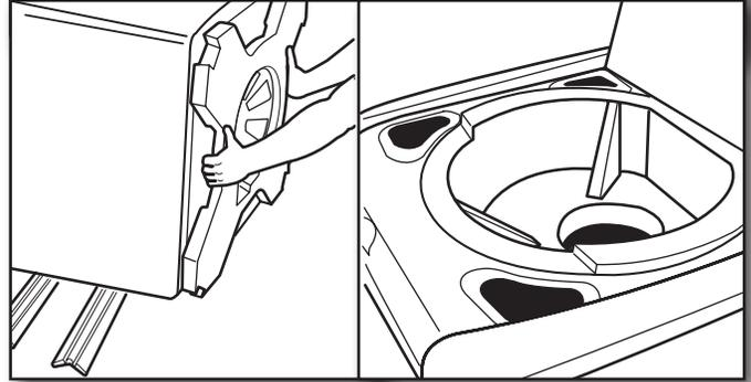
Place cardboard supports from shipping carton on floor behind washer for support. Secure the lid with tape. Using two or more people, tip the washer onto its back and place on cardboard supports. Remove foam shipping base. Then, set washer back upright, and remove the tape from the lid so that you can open the lid and remove the foam packing ring from the washer tub.
