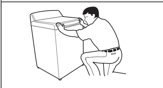
Move the washer to its final location. Rock the washer back and forth to check whether all four feet are stable and in firm contact with the floor. If the washer rocks, your model may be one that comes with 3 feet preset at the factory. It will be necessary to adjust the right front foot to level the washer. If all 4 feet were preset at the factory, minor adjustments may be needed to level the washer on your floor.
