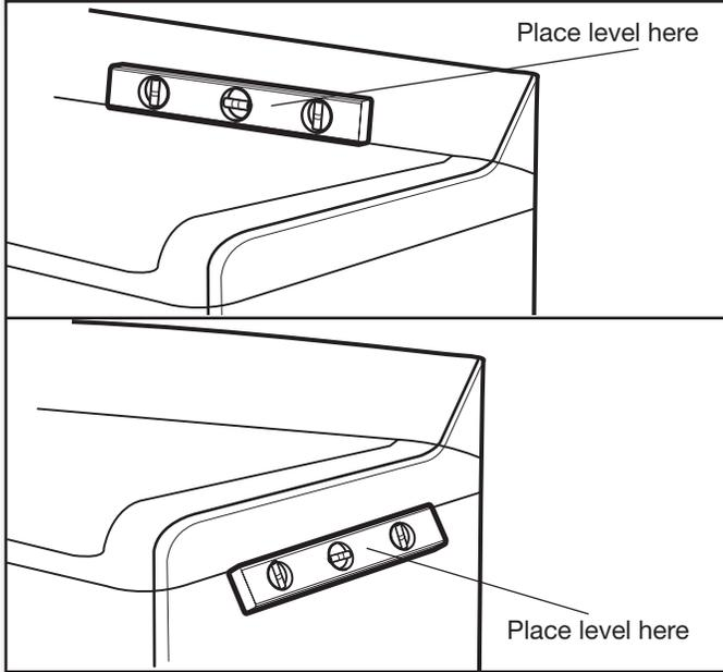
Check the levelness of the washer. First, place a level on the lid near the console. Then place the level on the side of the washer in the crease between the top of the washer and the cabinet.
