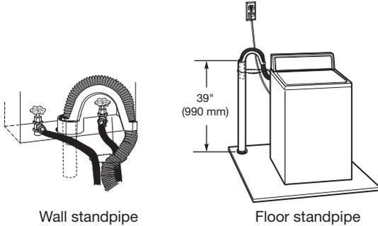
The standpipe drain requires a minimum diameter standpipe of 2" (51 mm). The minimum carry-away capacity can be no less than 17 gal. (64 L) per minute. A 2" (51 mm) diameter to 1" (25 mm) diameter standpipe adapter kit is available. See "Tools and Parts".
