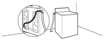
Floor drain system requires a Siphon Break Kit (Part Number 285834), 2 Connector Kits (Part Number 285835), and an Extension Drain Hose (Part Number 285863) that may be purchased separately. To order, please see toll-free phone numbers in your "Use and Care Guide." Minimum siphon break: 28" (710 mm) from bottom of washer. (Additional hoses may be needed.)
