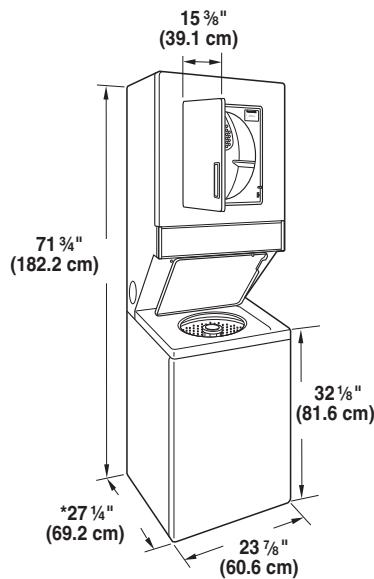
\* Most installations require a minimum 5" (12.7 cm) clearance behind the dryer for the exhaust vent with elbow.
