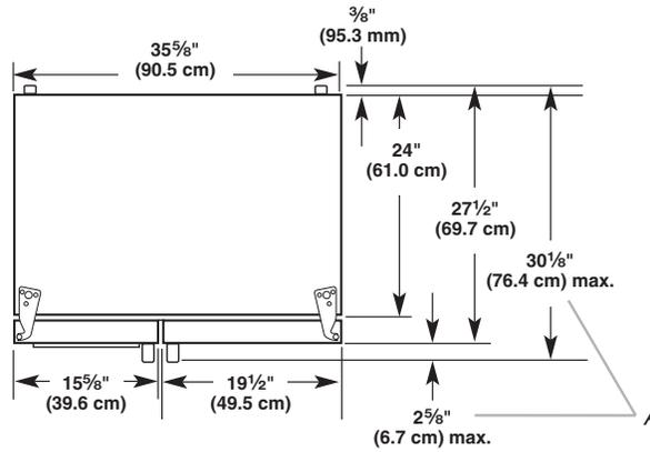
■ Height dimensions are shown with the leveling legs extended to the minimum height of 1/4" (6.35 mm) below the refrigerator.
