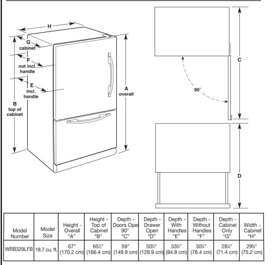
To ensure proper ventilation for your refrigerator, allow for a  $\frac{1}{2}$ " (1.25 cm) space on each side and at the top. Allow at least 1" (2.54 cm) between back of cabinet and the wall. If your refrigerator has an ice maker, make sure you leave some extra space at the back for the water line connections.
