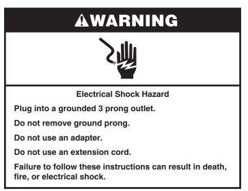
**Electrical:** A 115 V, 60 Hz, AC only 15 A or 20 A fused, grounded electrical supply is required. It is recommended that a separate circuit serving only your refrigerator be provided. Use an outlet that cannot be turned off by a switch. Do not use an extension cord.
