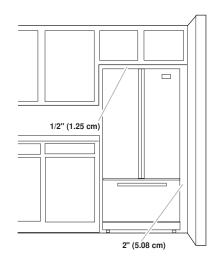
To ensure proper ventilation for your refrigerator, allow for a 1/2" (1.25 cm) of space on each side and at the top. Allow for a 1" (2.54 cm) space behind the refrigerator. If your refrigerator has an ice maker, allow extra space at the back for the water line connections. When installing your refrigerator next to a xed wall, leave a 2" (5.08 cm) minimum space between the refrigerator and wall to allow the door to swing open.
