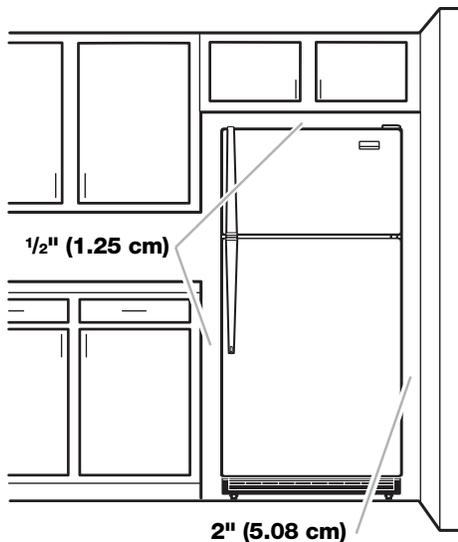
To ensure proper ventilation for your refrigerator, allow for a 1/2" (1.25 cm) space on each and between overhead cabinets and refrigerator top. Allow at least 1" (2.5 cm) between back of cabinet and the wall. If your refrigerator has an ice maker, make sure you leave some extra space at the back for the water line connections.
