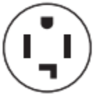
4-wire receptacle (14-30R)
