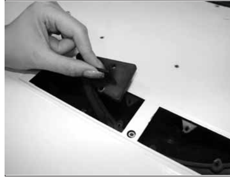
6. Remove (2) interior recirculating panels.
