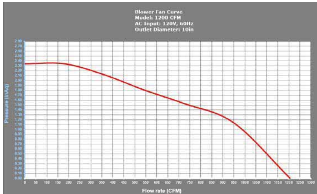
Dual Blower Fan Curve Diagram
